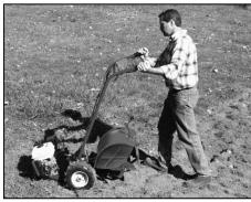
Figure 4-3: Find balance point before turning.
